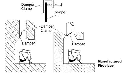
Figure 10 - Attaching Damper Clamp
